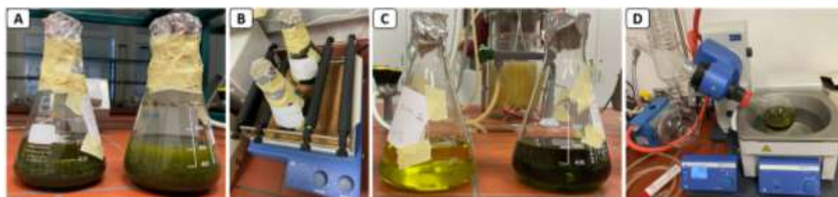
Figure 2. (A) Maceration mixture in solvents. (B) Mixture on the laboratory shaker. (C) Maceration mixture after filtration. (D) Evaporation of solvent on rotary evaporator.
