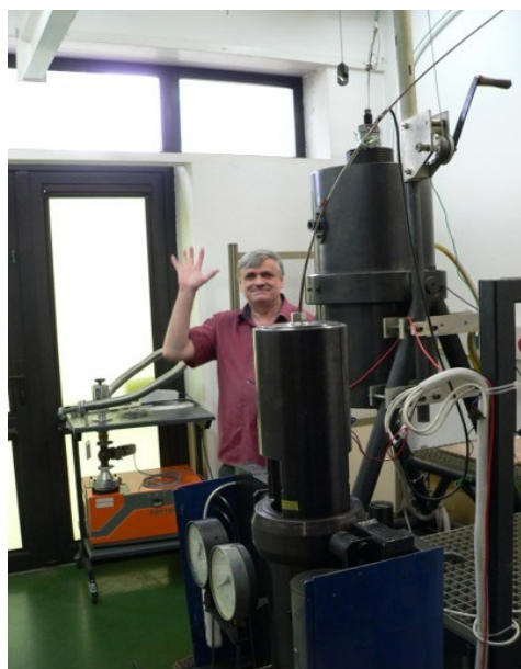
Figure 6. High-Pressure (up to 2.4 GPa), and High-Temperature processor ( > 1200 °C), with the pressure chamber volume V = 1 L, internal heater and gas (Nitrogen, Argon, Helium) as the medium transferring pressure. Available in IHPP PAS 'Unipress', Warsaw, Poland. The co-author of this report is saying 'Hello' in the picture.
