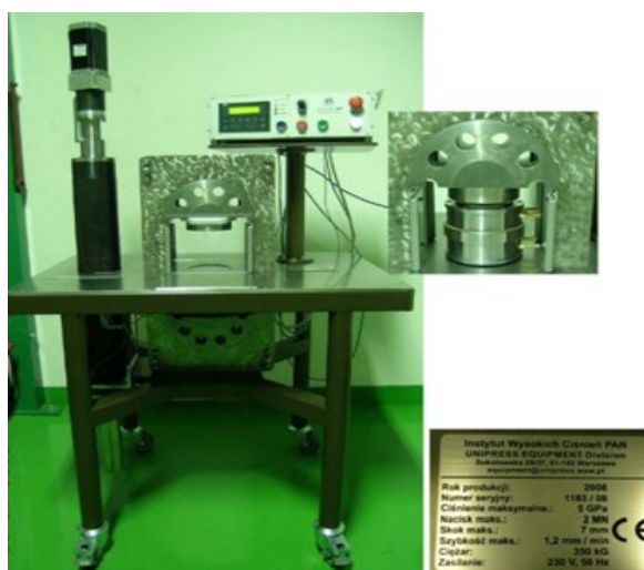
Figure 8. Anvil cell facility, made of superhard sintered carbide, working volume V \sim 1\text{ mL} , extreme pressures up to \sim 10\text{ GPa} . Available in IHPP PAS.
