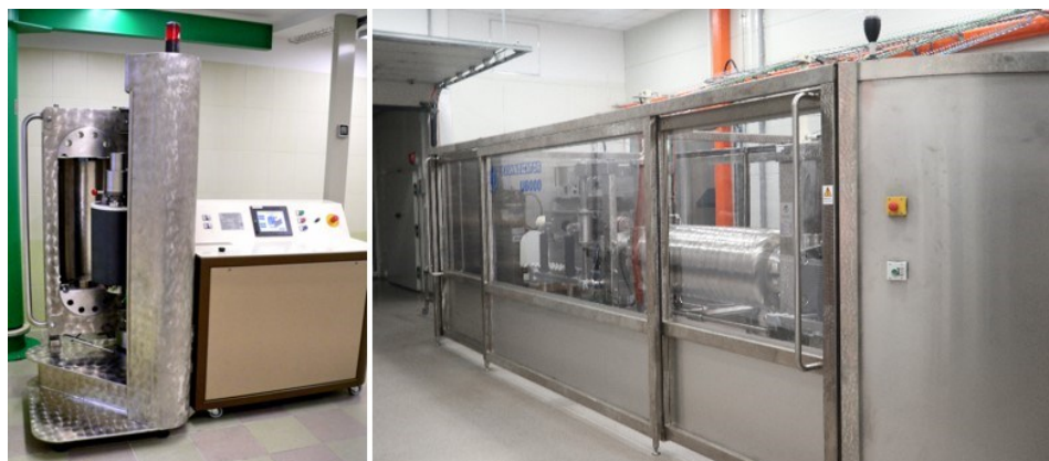
Figure 9. Processors for High Pressure Processing/Preservation (HPP) of foods, pharmaceuticals, or cosmeceuticals. Left: the lab-scale processor for pressures up to P = 600\text{ MPa} , -15\text{ }^{\circ}\text{C} < T < 90\text{ }^{\circ}\text{C} , V = 1.1\text{ L} . Right: the pilot (semi-industrial) scale HPP processor for pressures up to P = 600\text{ MPa} , and the pressure chamber volume V = 50\text{ L} . The facility is available in IHPP PAS 'Unipress', X-Press-Matter Lab, Warsaw, Poland ( https://young4softmatter.pl/ ).
