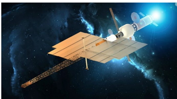
Figure 10. Nuclear Electric Propulsion (NEP) system for Space Ships, following National Aeronautics and Space Administration (NASA), (Atkinson, 2025). In the report, the link to metallic hydrogen 'fuel', given its unique properties, is considered.
